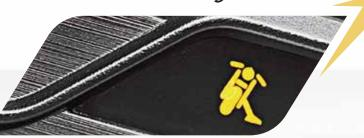
Adds to the safety of the rider. It cuts off the ignition if the vehicle is put in gear when the side stand is engaged.
